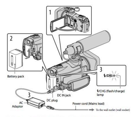
You can charge the "InfoLITHIUM" battery pack (V series) after attaching it to your camcorder.
